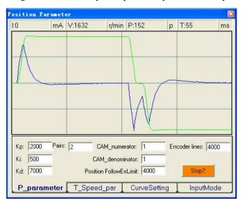
Figure 36: Position following error curve and velocity curve (Kp=2000, Ki=500 and Kd=7000)
