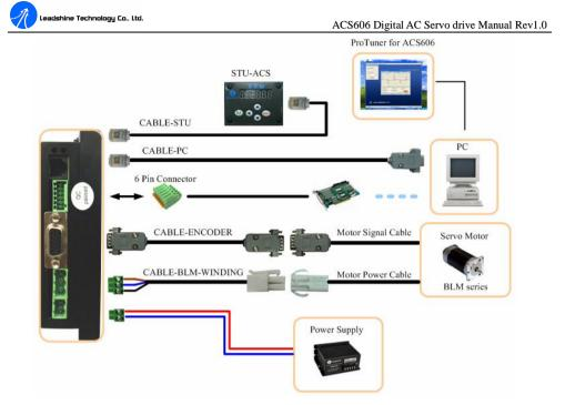
Figure 53: ACS606 accessories and connections with extended cable
