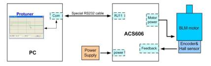
Figure 20: Configuration and connections before Tuning
