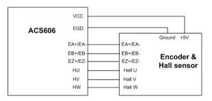
Figure 7: The ACS606 supplies the encoder directly
