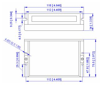
Figure 1: Mechanical specifications
