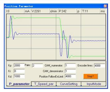
Figure 33: Position following error curve and velocity curve (Kp=2000, Ki=0 and Kd=1000)
