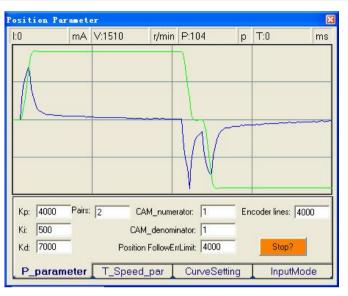
Figure 37: Position following error curve and velocity curve (Kp=4000, Ki=500 and Kd=7000)
