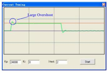
Figure 28: Response with High Kp of current-loop (Kp = 24000)
