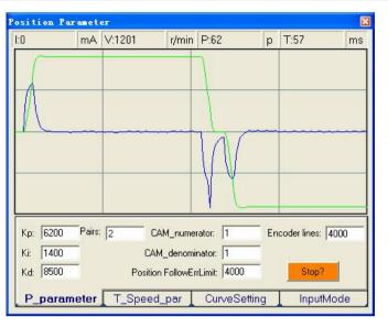
Figure 43: Position following error curve and velocity curve (Kp=6200, Ki=1400 and Kd=8500)
