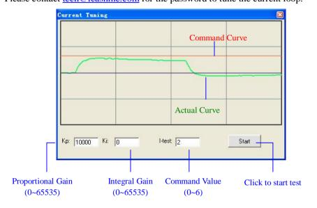
Figure 26: Current-loop tuning window
