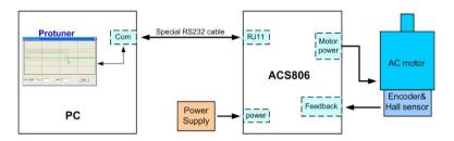
Figure 20: Configuration and connections before Tuning
