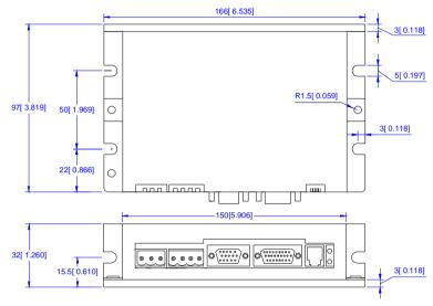
Figure 1: Mechanical specifications
