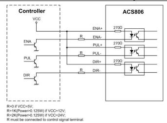
Figure 3: connections to controller with Common-Anode outputs
