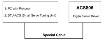
Figure 9: RS232 interface connection
