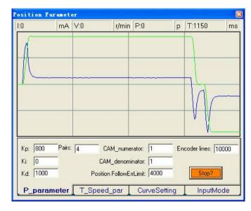
Figure 35: Position following error curve and velocity curve (Kp=800, Ki=0 and Kd=1000)
