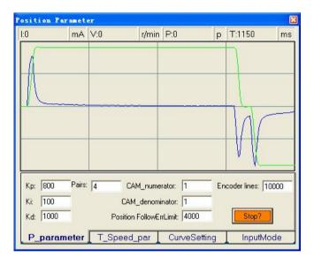
Figure 36: Position following error curve and velocity curve (Kp=800, Ki=100 and Kd=1000)
