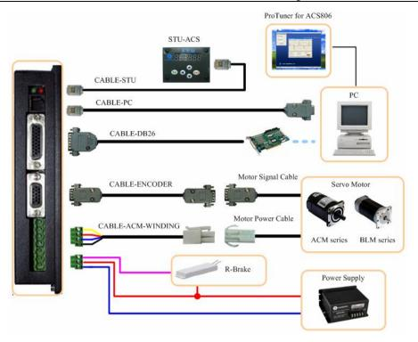
Figure 53: ACS806 accessories and connections with extended cable
