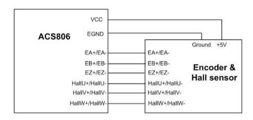
Figure 7: The ACS806 supplies the encoder directly
