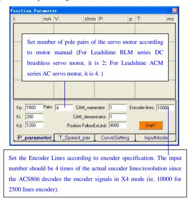
Figure 25: Software configuration before Tuning
