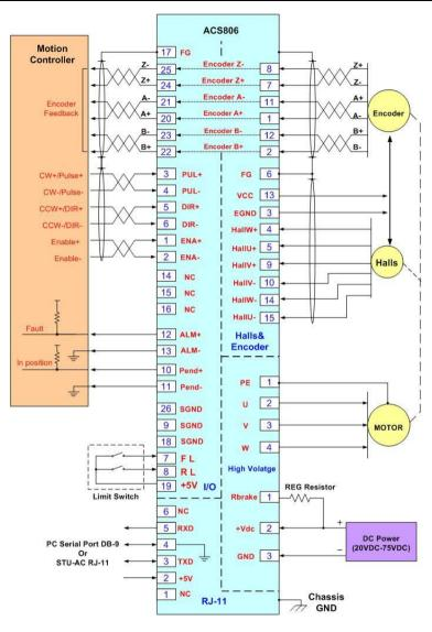
Figure 10: Typical connection of the ACS806
