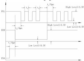
Figure 51: Sequence chart of control signals
