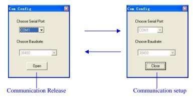
Figure 24: Establish and release series communication
