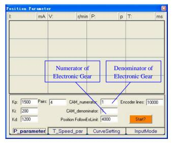
Figure 50: Electronic gear and position following error setting
