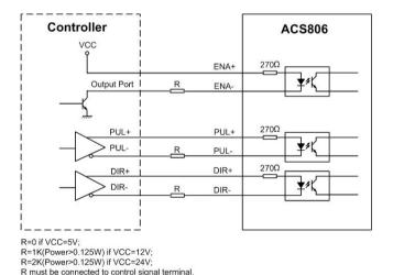
Figure 2: Connections to controller with differential outputs
