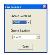
Figure 6-11: RS232 communication configuration window
