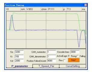
Figure 6-31: Position following error curve and velocity curve (Kp=3200, Ki=600 and Kd=4000)
