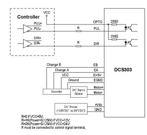
Figure 3-6: Typical connection (Differential control signal)
