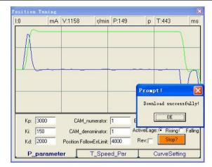
Figure 6-32: Position following error curve and velocity curve (Kp=3000, Ki=150 and Kd=2000)
