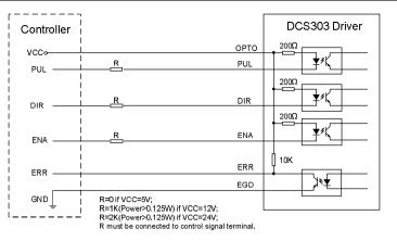
Figure 3-1: Connections to open-collector control signal (common-anode)
