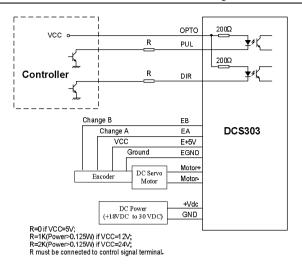
Figure 3-5: Typical connection (Open-collector control signal.)
