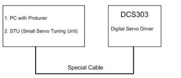
Figure 6-9: RS232 interface connection
