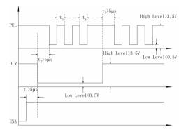
Figure14: Sequence chart of control signals
