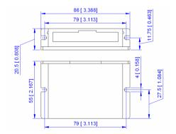
Figure 2-1: Mechanical specifications
