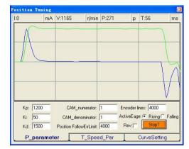
Figure 6-24: Position following error curve and velocity curve (Kp=1200, Ki=50 and Kd=1500)
