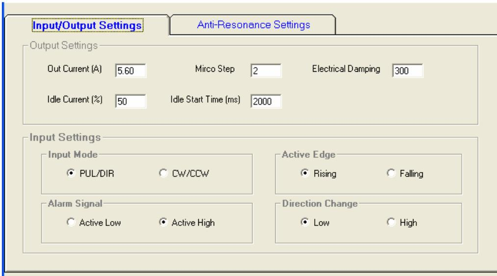
In most application, it is only required to the output current, micro step and input mode. Usually, the motor manufacturer states the RMS (root mean square) current in datasheet. Please refer to the hardware installation manual for how to set the output current.
