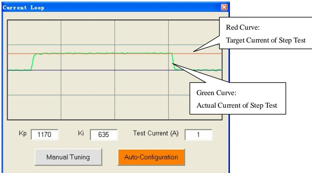
Click **Drive->Current Loop** to open the current loop tuning window. You can adjust the Kp (proportional gain) and Ki (integral gain) in this window. These parameters should be tuned before normal operation.
