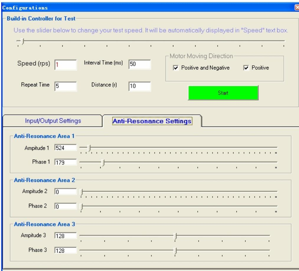
You can adjust the anti-resonance parameters in this window. The built-in controller can be assist anti-resonance tuning and self test.
