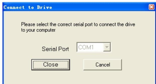
**Connect to Drive** window appears every time you open ProTuner. You can also open it by clicking **Communication>Connect To Drive** when the software is open. Select the serial port and click on the **Connect** button. The software will try to connect to the drive and read the settings. It may take several minutes. Please wait.
