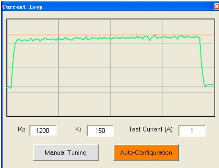
**Step 5:** The current loop tuning is basically finished. You can continue to adjust Kp and Ki for better performance. Now the updated **Kp** and **Ki** is just stored in the driver's RAM. They will be lost when we power off the driver. **Don't forget to click Drive->Download To Drive to store the changed value to the drive's nonvolatile memory.**
