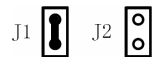
(b) J1 short circuit, J2 open circuit PUL/DIR mode and active at downward-falling edge
