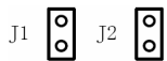
(a) J1, J2 open circuit PUL/DIR mode and active at upward-rising edge
