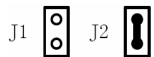
(c) J1 open circuit, J2 short circuit CW/CCW mode and active at high level (The fixed level)
