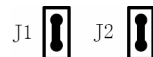
(d) J1, J2 short circuit CW/CCW mode and active at low level (The fixed level)
